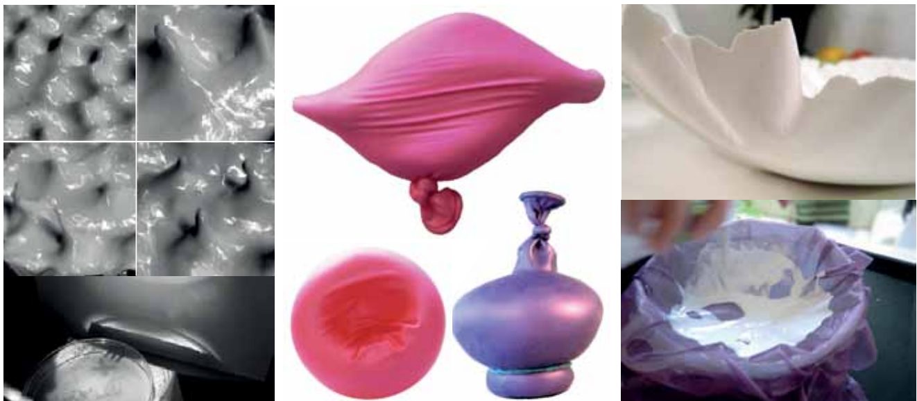
Figure 3: Examples of experimental physical modelling for exploring form ideas for a dinnerware project (student works), from left to right: (i) transmitting soundwaves through a liquid, (ii) using balloons & flour, and (iii) using plaster & cotton.
